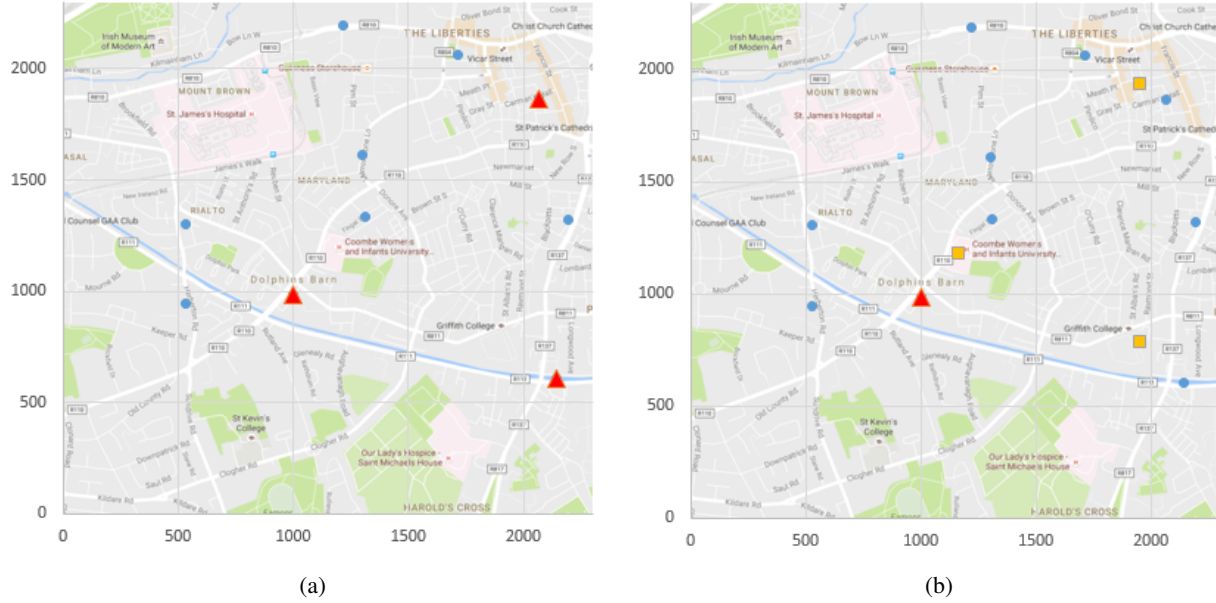
Fig. 4: Simulation scenario during the fourth period (i.e., from 90 to 120s) when considering (a) Traditional and (b) DSM approaches. Blue dots represent regular BSs and red triangles represent those that are receiving a great number of messages. Operational SCs are represented by yellow squares.
