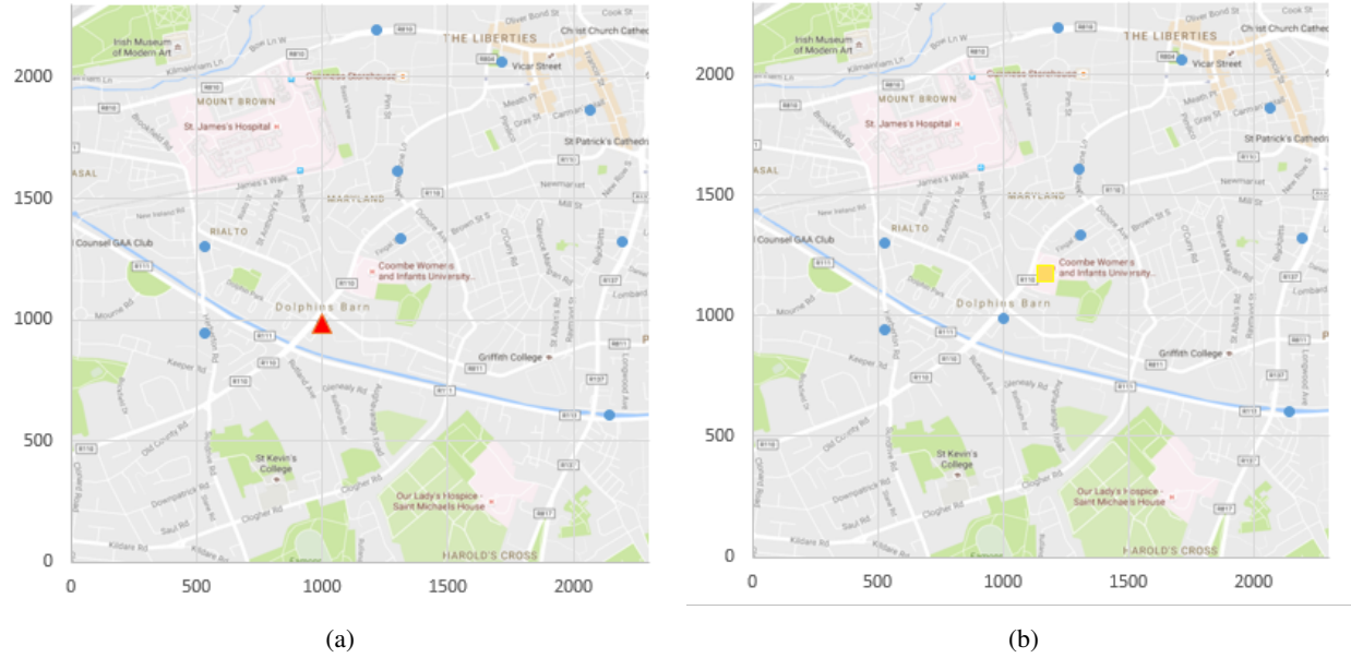
Fig. 2: Simulation scenario during the first time period (i.e., from 0 to 30s) when considering (a) Traditional and (b) DSM approaches. Blue dots represent regular BSs and red triangles represent those that are receiving a great number of messages. Operational SCs are represented by yellow squares.
