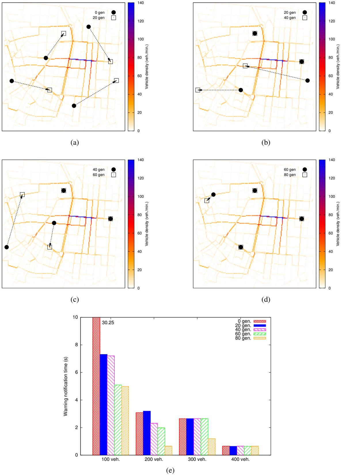
Fig. 3. Evolution of the deployment of 4 RSUS in the Madrid scenario using GARSUD: (a) after 20 generations, (b) after 40 generations, (c) after 60 generations, and (d) after 80 generations. The evolution of warning notification time for each vehicle density is shown in (e).
