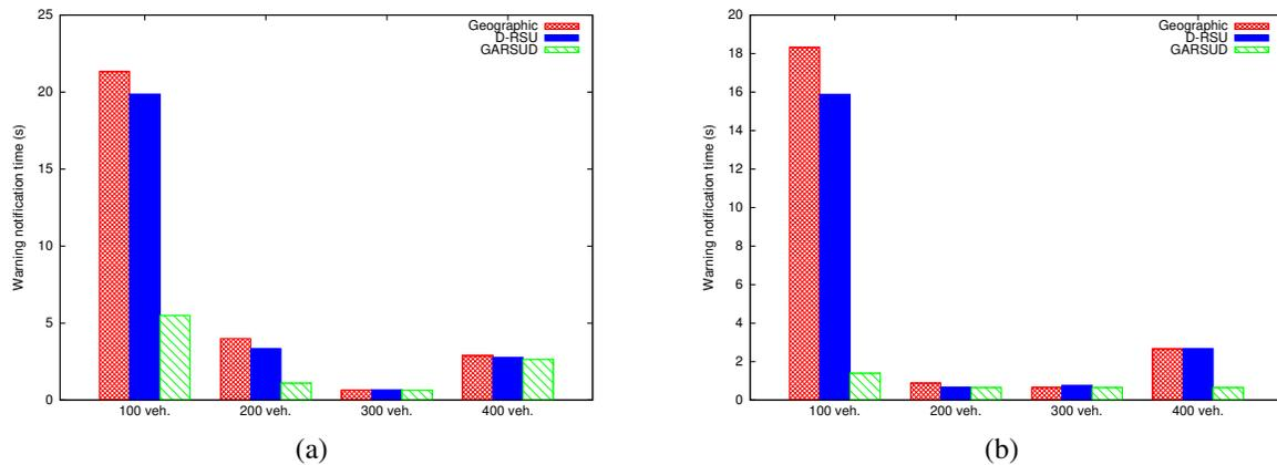
Fig. 5. Warning notification time in Madrid when varying the density of vehicles and deploying (a) 4 RSUs and (b) 9 RSUs.
