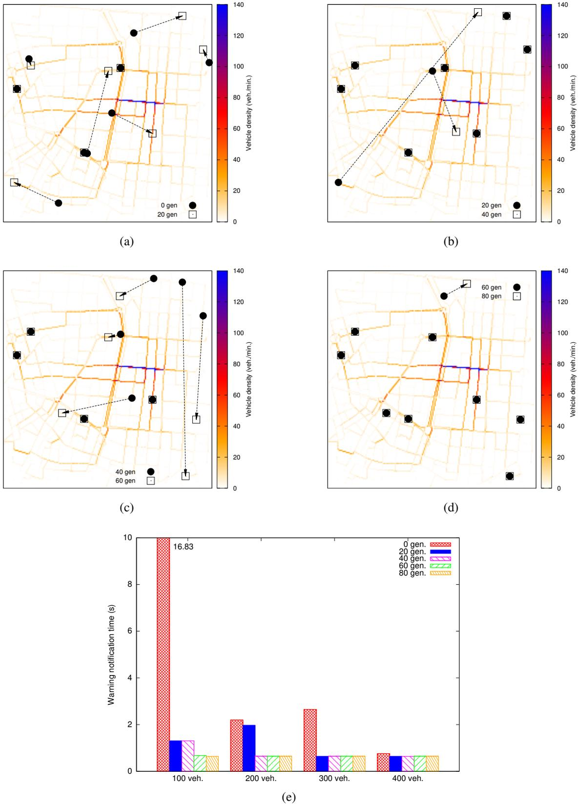
Fig. 4. Evolution of the deployment of 9 RSUS in the Madrid scenario using GARSUD: (a) after 20 generations, (b) after 40 generations, (c) after 60 generations, and (d) after 80 generations. The evolution of warning notification time for each vehicle density is shown in (e).
