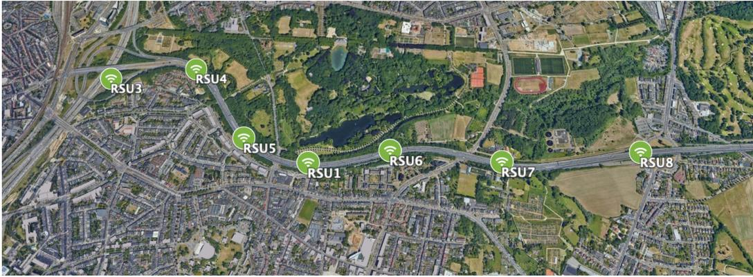
Fig. 2. The locations of the RSUs deployed along the E313 highway.
