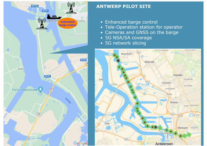
Fig. 1: A high-level overview of the Antwerp pilot site created for testing and validating automated barge control, with an indicated 4G/5G signal coverage on the sailing route (green indicating good signal quality).
