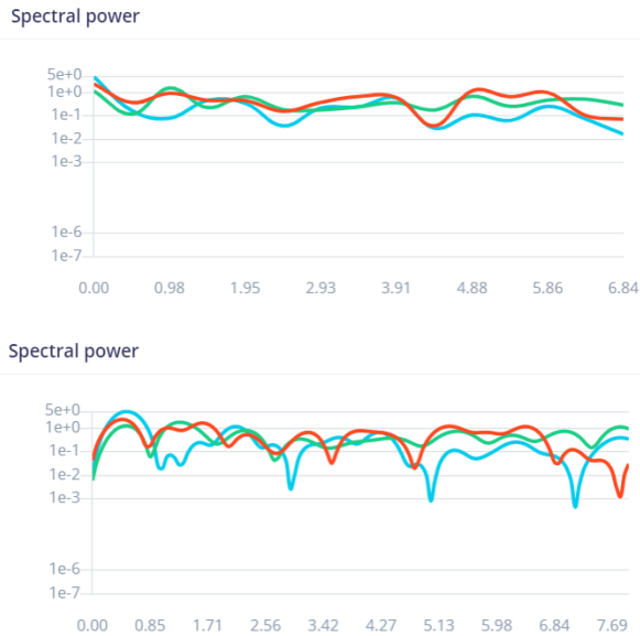
Fig. 5: The spectral power graph generated using FFT of variable length, the top figure contains 128 points, the bottom one contains 1024 points. The x-axis contains the frequency in Hz and the y-axis contains the power for that frequency.
