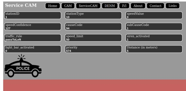
Fig. 2. Displaying the type of special vehicle that is sending CAMs
