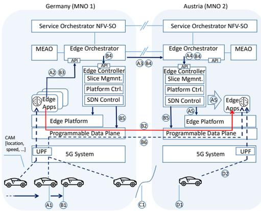
Fig. 2: Smart EdgeApps and TEB for service continuity.
