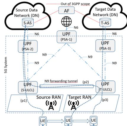
Fig. 1: Forwarding between ULCLs during network relocation [3].
