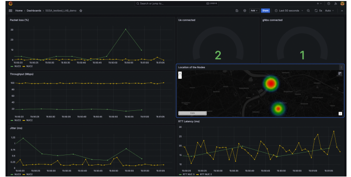
Fig. 3: Real-Time dashboard for traffic monitoring within the 5G SA network.
