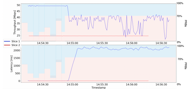
Fig. 4: Throughput and one-way latency behavior. In the background is shown the allocation of PRBs.
