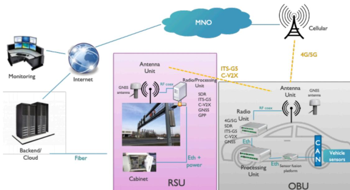
Figure 8 – Smart Highway Architecture
