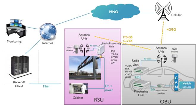
Fig. 2. Smart Highway Architecture
