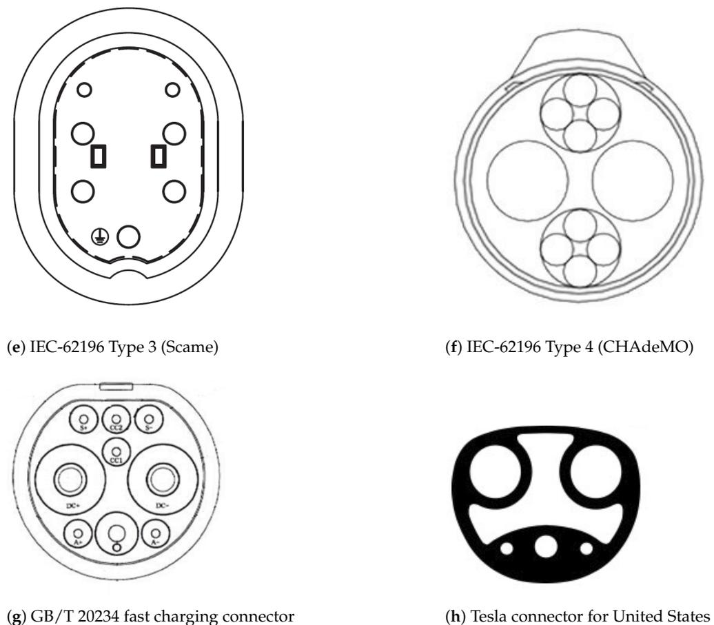
**Figure 7.** EV Connectors considered by the different standards [77–79].
