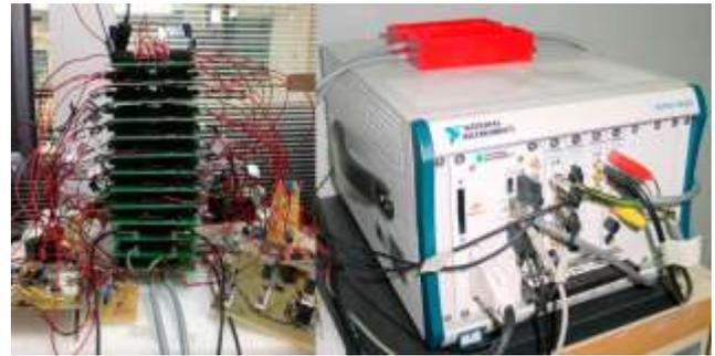
**Figure 1: Hardware of the VISIR system installed at UNED: PXI chassis in which the instruments and equipment cards from National Instruments are installed; and a relay switching matrix in which the components are plugged.**
