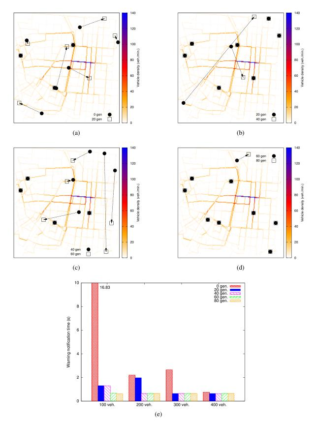
Fig. 4. Evolution of the deployment of 9 RSUS in the Madrid scenario using GARSUD: (a) after 20 generations, (b) after 40 generations, (c) after 60 generations, and (d) after 80 generations. The evolution of warning notification time for each vehicle density is shown in (e).
