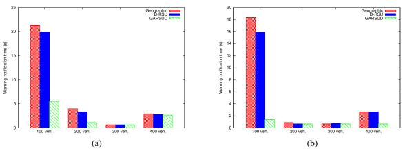
Fig. 5. Warning notification time in Madrid when varying the density of vehicles and deploying (a) 4 RSUs and (b) 9 RSUs.
