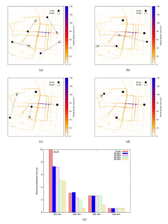
Fig. 3. Evolution of the deployment of 4 RSUS in the Madrid scenario using GARSUD: (a) after 20 generations, (b) after 40 generations, (c) after 60 generations, and (d) after 80 generations. The evolution of warning notification time for each vehicle density is shown in (e).
