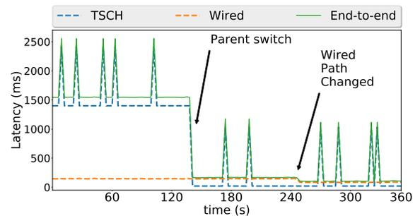
Fig. 3. Latency readings from node 4. First, a parent switch occurs in the 6TiSCH network. Secondly, the wired topology is modified as well to minimize the overall end-to-end latency.
