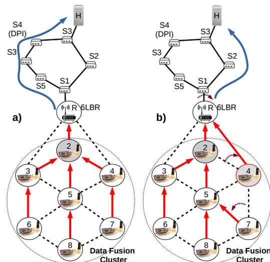
Fig. 1. In (a), the 6TiSCH network is aggregating data at node 2. In (b), network is end-to-end reconfigured to achieve lowest latency in node 4. Also, node 7’s next hop is changed to continue aggregating its readings at node 2.
