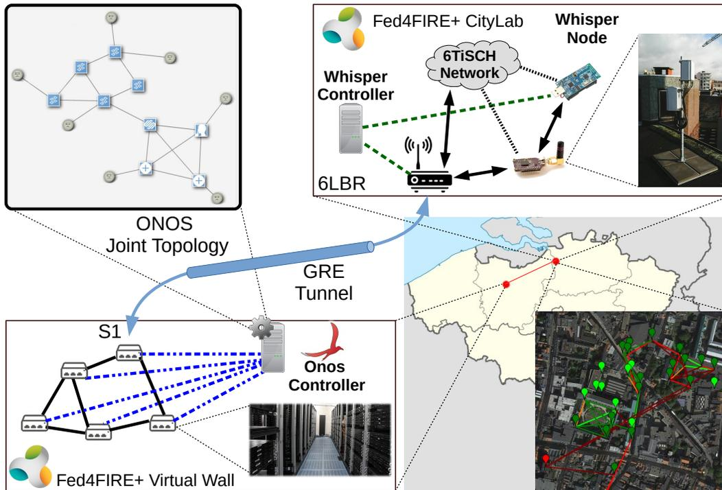
Fig. 2. Architecture of the multi-domain network deployed in two different Fed4FIRE+ testbeds to provide end to end control.
